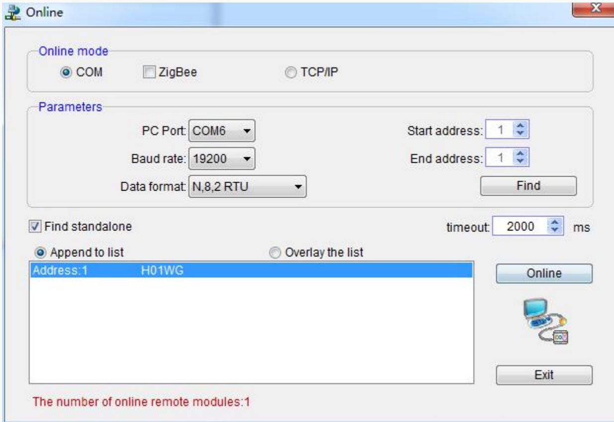
If there is only one plc on the 485 port, then you can use “find standalone”. If there are many, set the start address and stop address, so that all the machines on the 485 port can be found and the parameters are configured. Click exit to enter the configuration interface.
