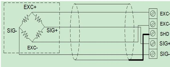
6-wire sensor and instrument connection:
