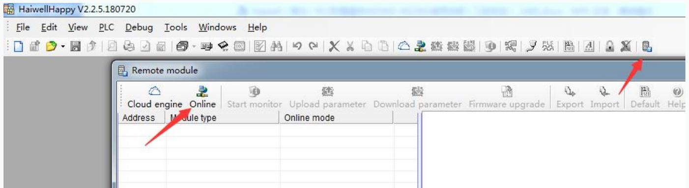
The default address of the module is 1 with format 19200, N 82 RTU, and the online success is as follows:
