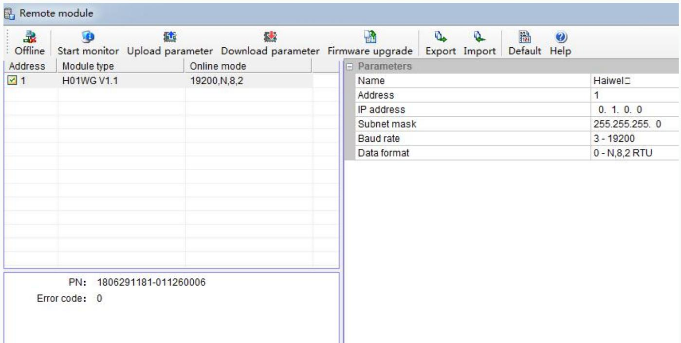
In the communication parameter area, we can change the module's name, address, baud rate and data format and other communication parameters, and then download it after modification.
