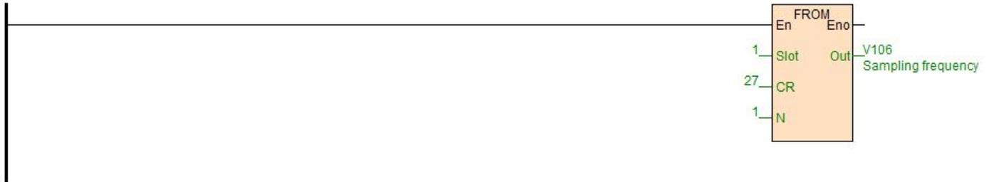
//Network 3 Set the sampling frequency 0-6.25HZ, 1-12.5HZ, 2-25HZ, 3-50HZ, 4-100HZ, 5-200HZ, 6-500HZ, 7-1000HZ
